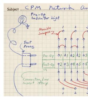
cal analogy of a project schedule. The Indicator Circuit was used to probe the plugboard, entries were made into a worksheet, and the schedule was then manually recalculated. With the help of Stanford's Electronics Lab, Fondahl constructed the more sophisticated Project Network Analyzer in 1964.
